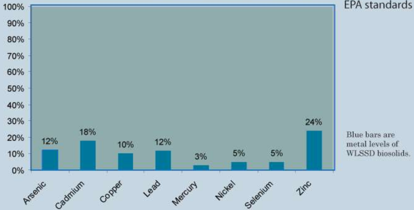
WLSSD biosolids metals as percentage of strictest U.S. EPA standards for each application
