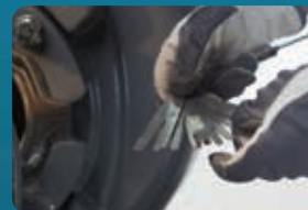
Simplified impeller check and adjustment with roll back cart and telescopic inlet
