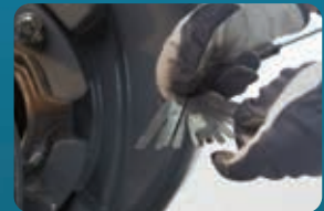
Simplified impeller check and adjustment with roll back cart and telescopic inlet
